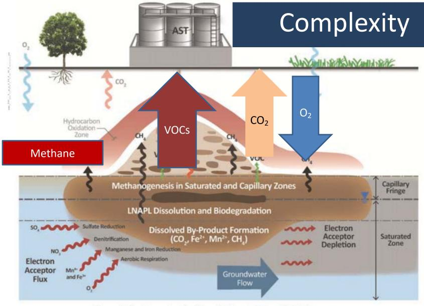
Figure 2-1—Conceptualization of Saturated Zone NSZD Processes
