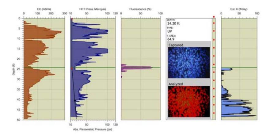
Figure 6: Graphs left to right: Soil EC, HPT pressure (formation permeability) along with absolute piezometric pressure (secondary axis), UV percent area Fluorescence, saved UV image from 24.20ft, and estimate hydraulic conductivity (estimated K).
